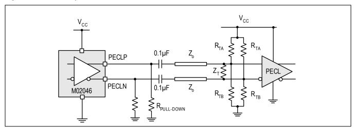
Figure 4-7. DC-Coupled PECL Termination
