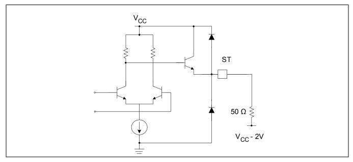
Figure 3-5. CMOS ST (M02046-15) and LOS (M02046-15 and M02046-25) Output
