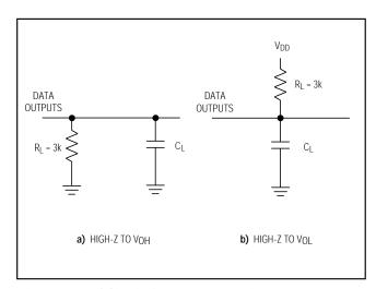
Figure 1. Load Circuits for Data-Access Time Test
