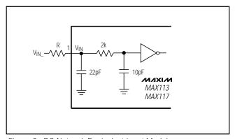
Figure 9. RC Network Equivalent Input Model
