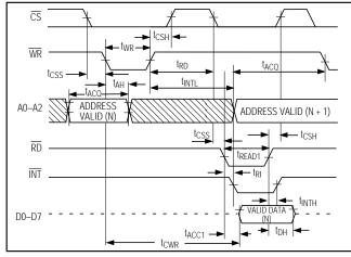
Figure 5. Write-Read Mode Timing (tRD < tINTL) (Mode = 1)
