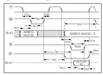
Figure 4. Write-Read Mode Timing ( $t_{RD} > t_{INTL}$ ) (Mode = 1)
