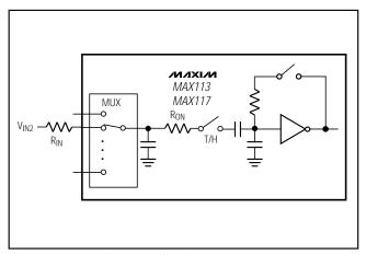
Figure 8. Equivalent Input Circuit
