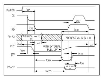
Figure 3. Read Mode Timing (Mode = 0)
