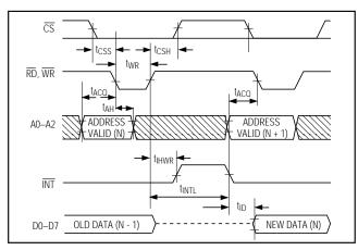
Figure 6. Pipelined Mode Timing ( $\overline{WR} = \overline{RD}$ ) (Mode = 1)
