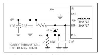
Figure 7c. Input Not Referenced to GND
