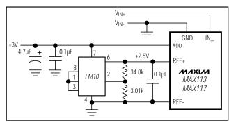
Figure 7b. External Reference, 2.5V Full Scale
