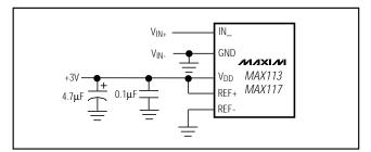
Figure 7a. Power Supply as Reference
