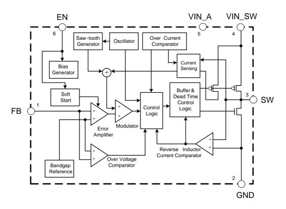
Figure 3. Functional Block Diagram of AUR9718B
