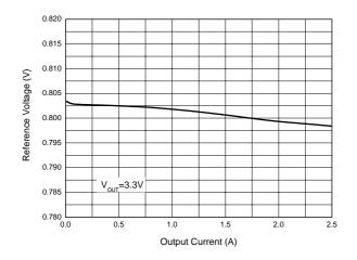
Figure 14. Reference Voltage vs. Output Current
