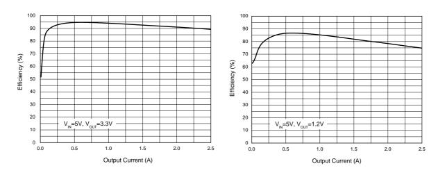
Figure 4. Efficiency vs. Output Current
