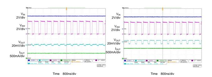
Figure 16.  $V_{OUT}$  Ripple ( $V_{IN}$ =5V,  $V_{OUT}$ =3.3V,  $I_{OUT}$ =500mA)
