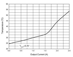
Figure 15. Temperature vs. Output Current
