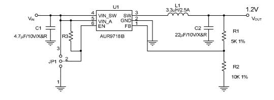
Figure 31. The Evaluation Board Schematic
