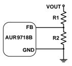
Figure 30. Setting the Output Voltage
