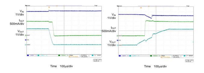
Figure 28. OVP Function  $(V_{IN}=5V \text{ to } 6V)$
