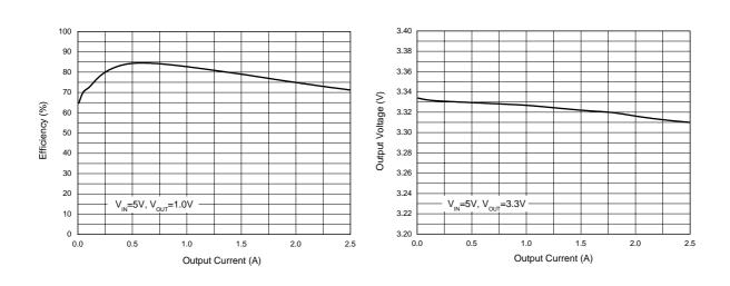
Figure 6. Efficiency vs. Output Current
