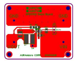
Figure 32. Top Layer for Demo Board
