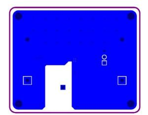
Figure 33. Bottom Layer for Demo Board
