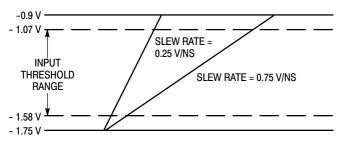
Figure 6. ECL Dispersion Test Input Conditions
