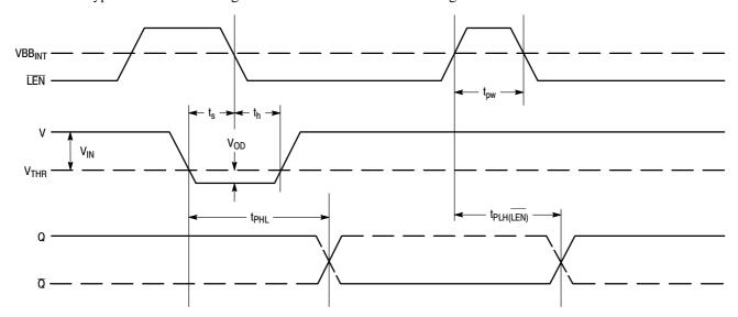
Figure 5. Input/Output Timing Diagram
