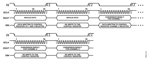
Figure 24. Configuring a Conversion and Read with the AD7298-1, Numerous Channels Selected for Conversion
