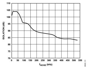
Figure 11. Channel-to-Channel Isolation,  $f_{IN} = 50 \text{ kHz}$
