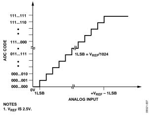
Figure 22. Straight Binary Transfer Characteristic
