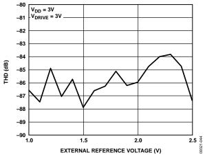
Figure 14. THD vs. Reference Voltage
