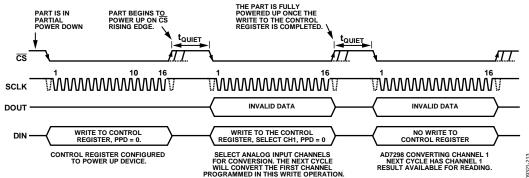
Figure 27. Partial Power-Down Mode of Operation
