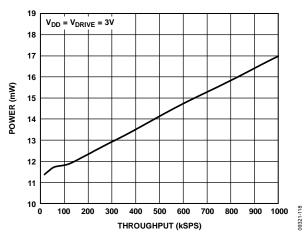
Figure 17. Power vs. Throughput in Normal Mode with  $V_{\rm DD} = 3 \text{ V}$
