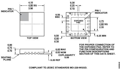
Figure 29. 20-Lead Lead Frame Chip Scale Package [LFCSP\_WQ] 4 mm × 4 mm Body, Very, Very Thin Quad (CP-20-8) Dimensions shown in millimeters
