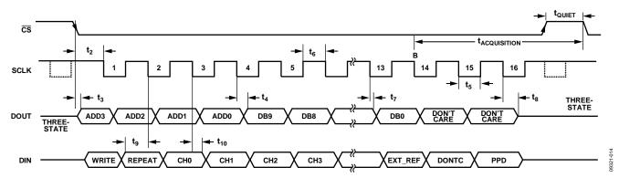
Figure 28. Serial Interface Timing Diagram
