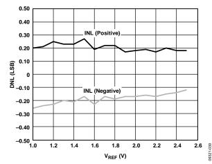
Figure 7. DNL vs.  $V_{REF}$
