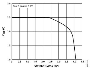
Figure 9.  $V_{REF}$  vs. Reference Output Current Drive
