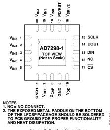
Figure 2. Pin Configuration
