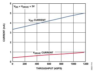
Figure 16. Average Supply Current vs. Throughput Rate
