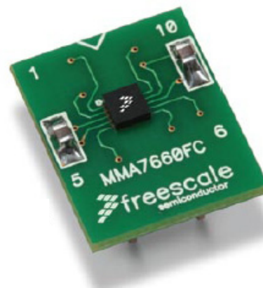
Figure 2. MMA7660FC Dip Board
