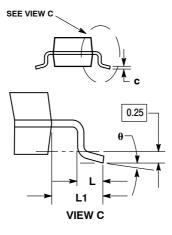
NOTES: 1. DIMENSIONING AND TOLERANCING PER ANSI Y14.5M, 1982. 2. CONTROLLING DIMENSION: INCH
