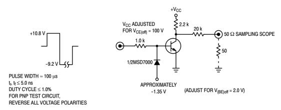
Figure 9. Switching Time Test Circuit
