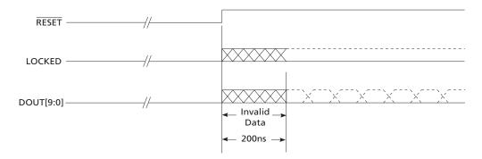
Figure 3-20: Reset Timing
