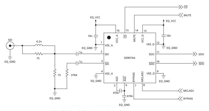
NOTE: All resistors in Ohms, capacitors in Farads, and inductors in Henrys, unless otherwise noted.
