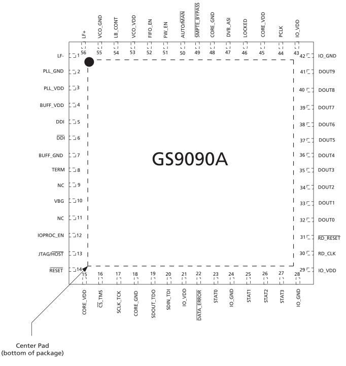
Figure 1-1: Pin Assignment
