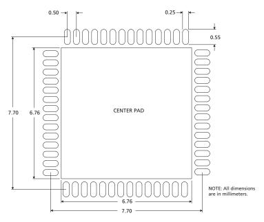
The Center Pad of the PCB footprint should be connected to the CORE\_GND plane by a minimum of 25 vias.
