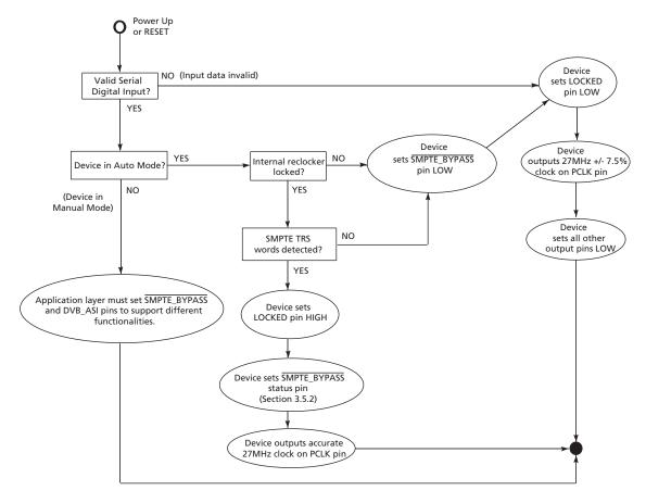
Figure 3-2: Lock Detection Process
