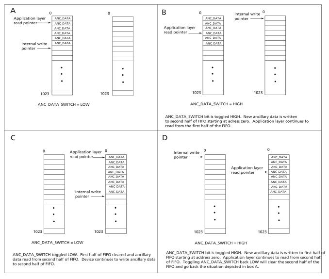
NOTE: At least 1100 PCLK cycles must pass between toggles of the ANC\_DATA\_SWITCH bit. The bit must be toggled at a point where no extraction is occuring (i.e. the ANC signal is LOW).
