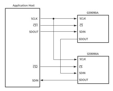
Figure 3-15: GSPI Application Interface Connection
