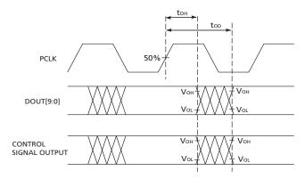
Figure 3-13: PCLK to Data & Control Signal Output Timing
