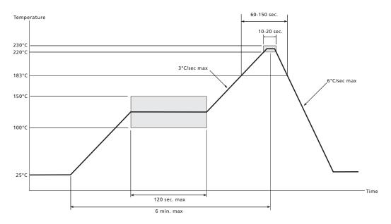
Figure 6-3: Standard Eutectic Solder Reflow Profile
