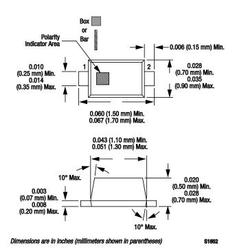
Figure 8. SC-79 Package Dimension Drawing
