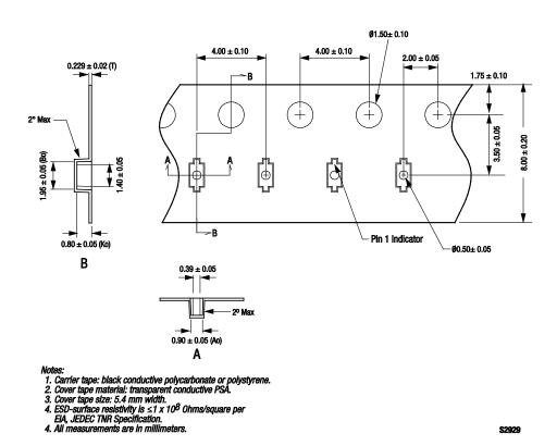
Figure 9. SC-79 Tape and Reel Dimensions
