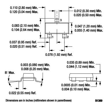
Figure 12. SOT-23 Package Dimension Drawing
