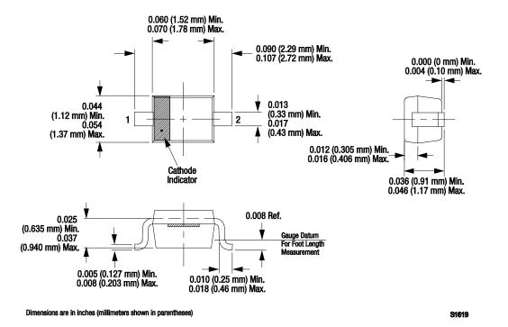
Figure 10. SOD-323 Package Dimension Drawing
