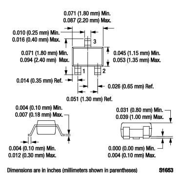
**Figure 6. SC-70 Package Dimension Drawing**
