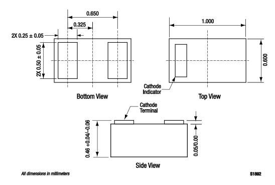
Figure 14. SOD-882 Package Dimension Drawing
