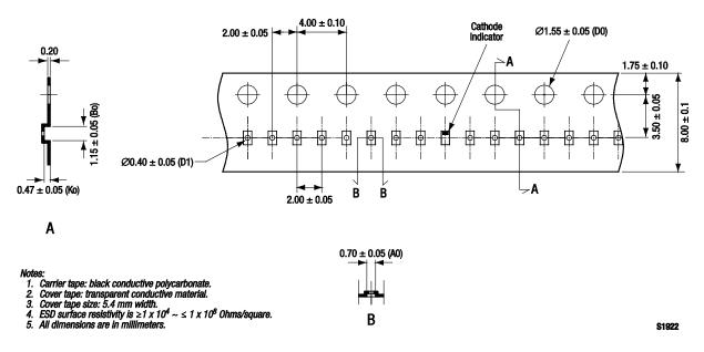
Figure 15. SOD-882 Tape and Reel Dimensions
