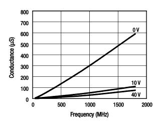
**Figure 5. Conductance vs Frequency and Reverse Voltage**
