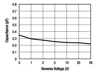
Figure 4. Capacitance vs Reverse Voltage (1 MHz to 1 GHz)
