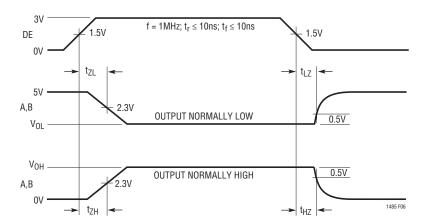
Figure 6. Driver Enable and Disable Times
