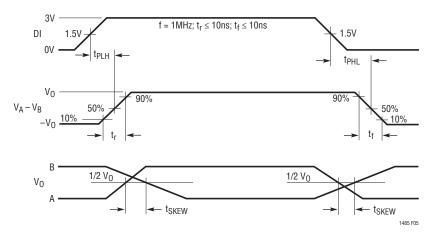
Figure 5. Driver Propagation Delays
