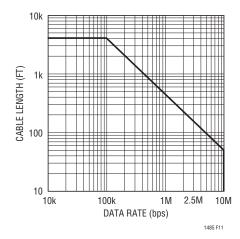
Figure 11. Cable Length vs Data Rate
