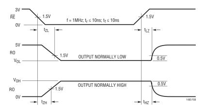
Figure 8. Receiver Enable and Disable Times
