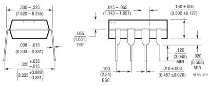
NOTE: 1. DIMENSIONS ARE  $\frac{\text{INCHES}}{\text{MILLIMETERS}}$
