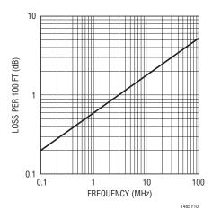
Figure 10. Attenuation vs Frequency for Belden 9481
