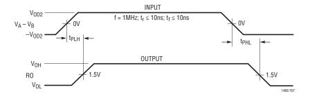
Figure 7. Receiver Propagation Delays
