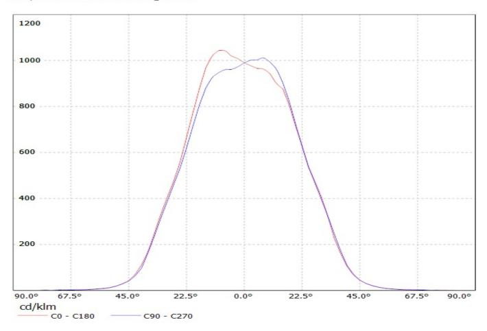
Luminaire: Ledil Oy CN12643\_LENINA-W-DL (Cree CXA20 698Im @ 250mA) Efficiency=78% Lamps: 1 x Cree CXA20 698Im @ 250mA
