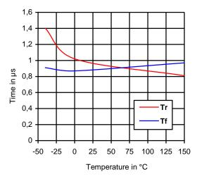
Figure 11: Current shutdown vs. temperature
