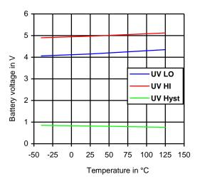
Figure 7: Under voltage parameters vs. temperature
