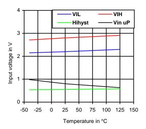
Figure 5: Input parameters vs. temperature
