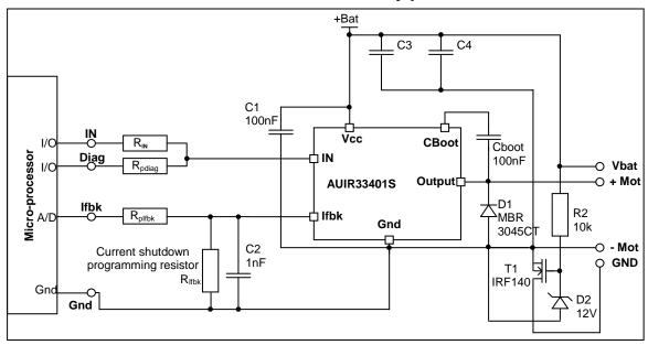
Figure 1: Recommended schematic
