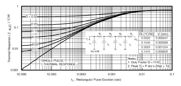
Figure 17: Transient thermal impedance vs. time
