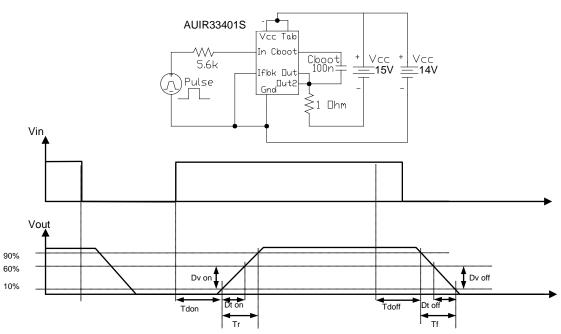
Figure 4: Switching time test circuit
