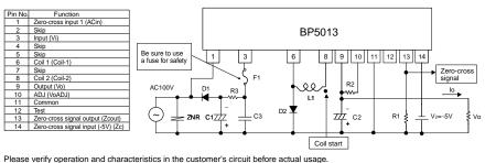
Ensure that the load current does not exceed the maximum rating.
