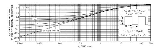
Figure 11. Transient Thermal Response Curve.
