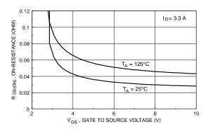
Figure 3. On-Resistance Variation with Temperature.
