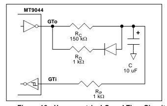
Figure 12 - Unsymmetrical Guard Time Circuit
