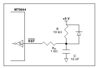
Figure 14 - Power-Up Reset Circuit
