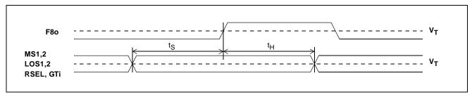
Figure 22 - Input Controls Setup and Hold Timing
