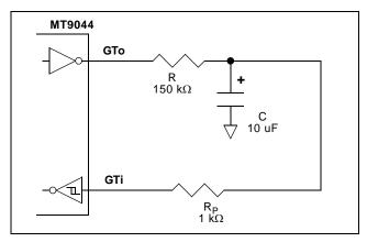
Figure 11 - Symmetrical Guard Time Circuit
