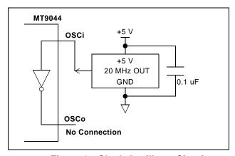
Figure 9 - Clock Oscillator Circuit
