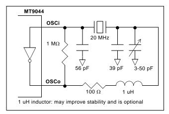
Figure 10 - Crystal Oscillator Circuit
