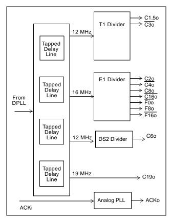
Figure 5 - Output Interface Circuit Block
