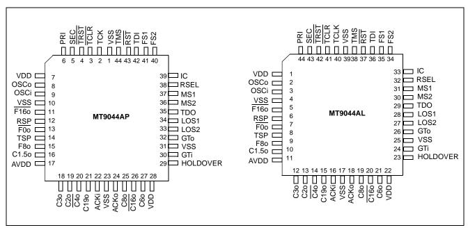
Figure 2 - Pin Connections
