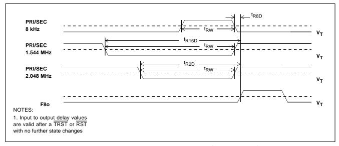
Figure 19 - Input to Output Timing (Normal Mode)
