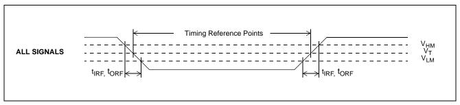
Figure 18 - Timing Parameter Measurement Voltage Levels
