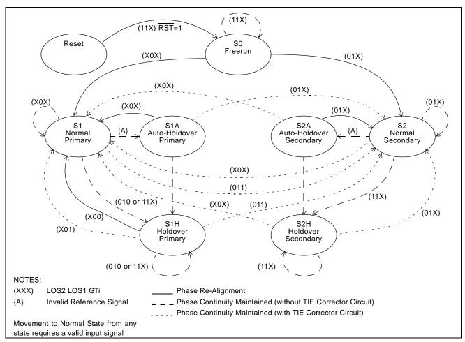
Figure 8 - Automatic Control State Diagram
