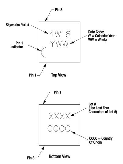
Figure 12. Typical Part Markings (Top View)
