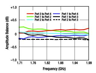
Figure 6. Amplitude Balance vs Frequency
