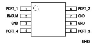
Figure 2. PD4W18-59LF Pinout – 8-Pin MSOP-8 (Top View)
