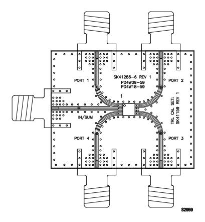
Figure 9. PD4W18-59LF Evaluation Board Assembly Drawing
