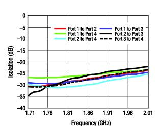
**Figure 5. Isolation vs Frequency**
