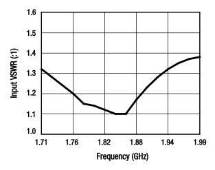
**Figure 7. Input VSWR vs Frequency**
