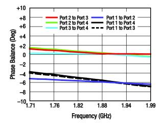
Figure 8. Phase Balance vs Frequency
