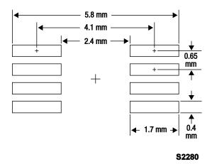
Figure 11. PD4W18-59LF PCB Layout Footprint
