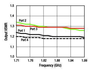
**Figure 4. Output VSWR vs Frequency**
