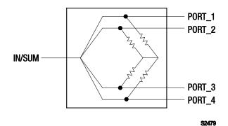
Figure 1. PD4W18-59LF Block Diagram
