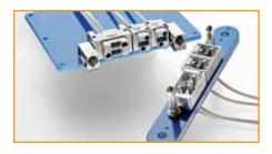
TE Connectivity's (TE) Ruggedized Optical Backplane interconnect system provides a high-density, blind-mate optical interconnect in a backplane/daughtercard configuration. The fiber optic ribbon cable interconnect feeds through the backplane to removable system modules using MT ferrules.
