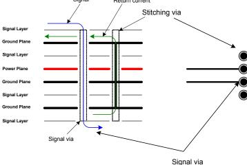
Figure 2. Return current path utilizing stitching vias
