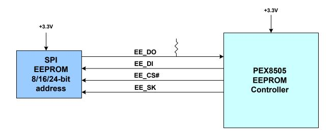
Figure 4. PEX 8505 SPI EEPROM Interface
