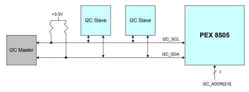
Figure 5. I2C bus connectivity
