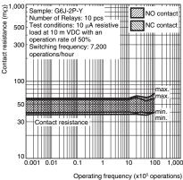
The tests were conducted at an ambient temperature of 23°C.
