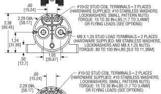
MOUNTING HARDWARE (NOT SUPPLIED: 2 X M5 BOLT 2 X M5 LOCKWASHER 2 X M5 NARROW WASHER) TORQUE: 15 TO 30 IN-LBS [1.7 TO 3.4NM]
