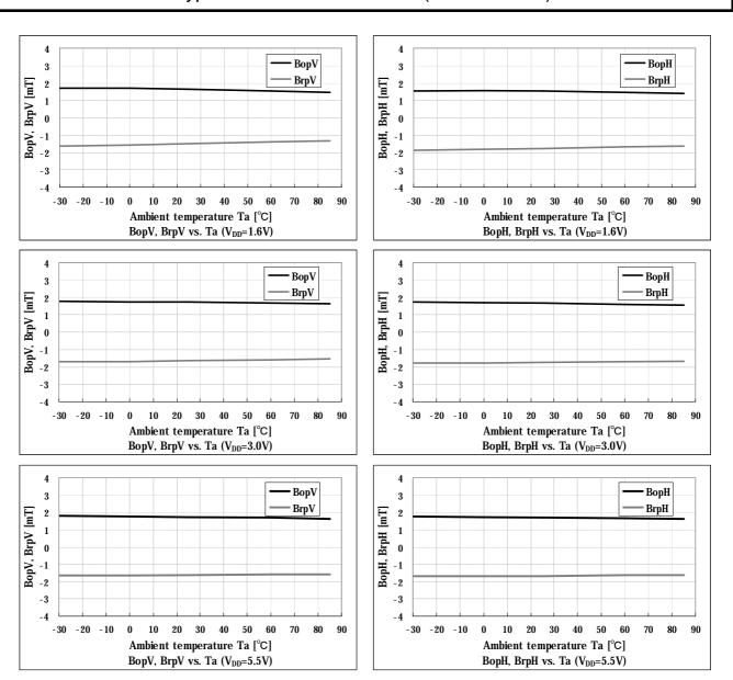
Figure 6. Temperature dependence of sensitivity
