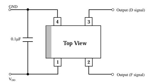
Figure 10. Recommended external circuit
