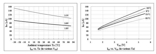
Figure 7. Temperature dependence of current consumption
