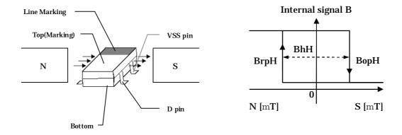
Figure 3. Switching behavior of internal signal B when horizontal magnetic field is applied
