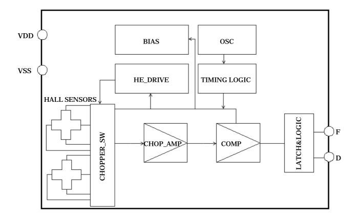
Figure 1. Block diagram
