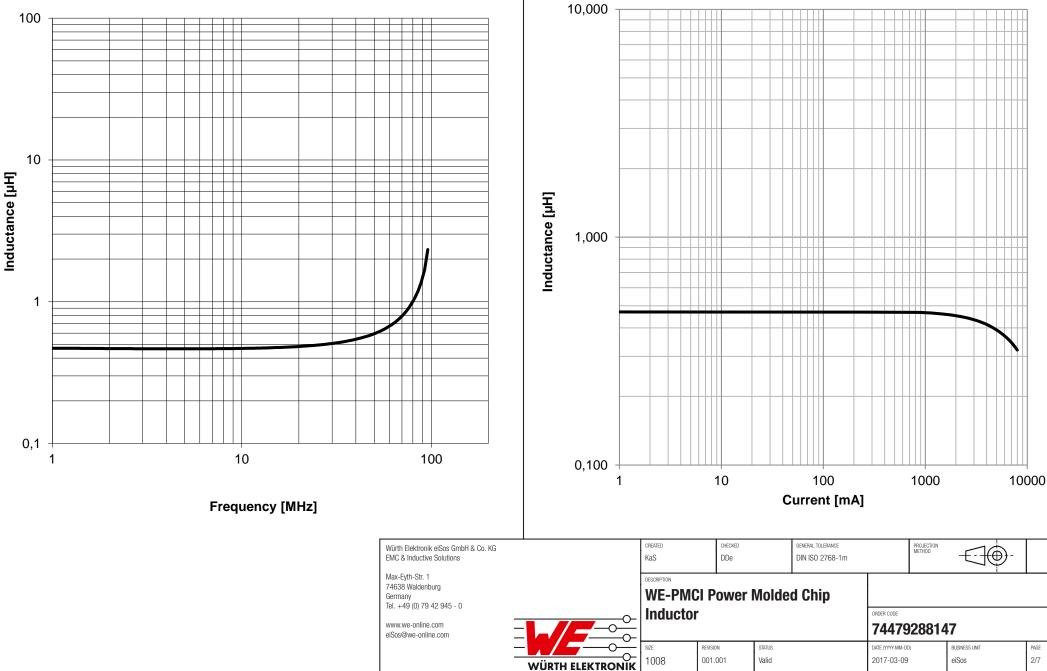
**Typical Inductance vs. Frequency Characteristics:**
