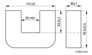
U cores are supplied as single units. The  $A_L$  value in the table applies to a core set comprising two ungapped cores.
