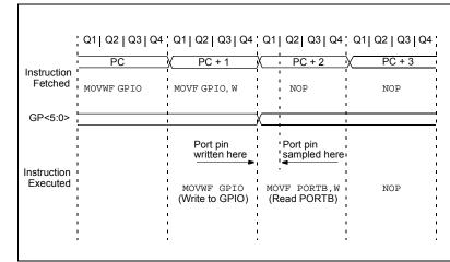
This example shows a write to GPIO followed by a read from GPIO.
