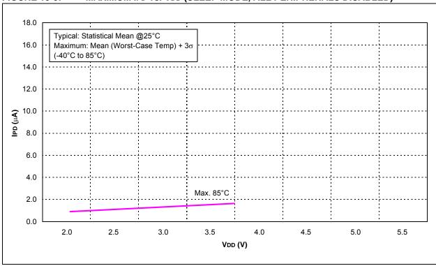
FIGURE 13-6: TYPICAL WDT IPD vs. VDD
