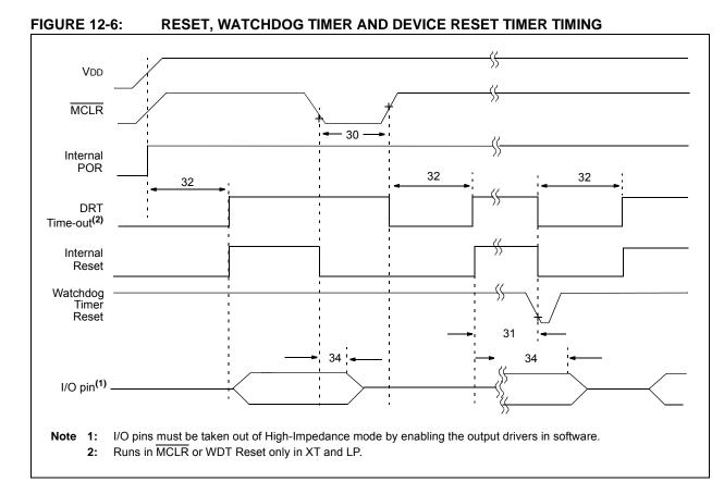
TABLE 12-7: RESET, WATCHDOG TIMER AND DEVICE RESET TIMER – PIC12F529T48A
