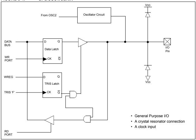
FIGURE 6-5: GP3 (WITH WEAK PULL-UP AND WAKE-UP ON CHANGE)
