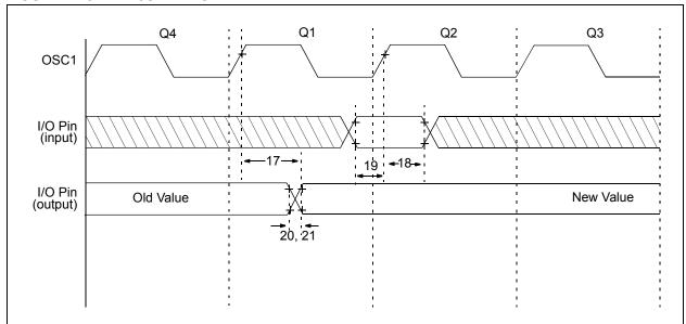
Note: All tests must be done with specified capacitive loads (see data sheet) 50 pF on I/O pins and CLKOUT.
