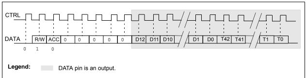
Note 1: When reading the Configuration register, 64 clock cycles on the CTRL pin must be issued, shifting out on the DATA pin the 13 Configuration bits, plus 43 internal test bits. Reading only the 13 Configuration bits is not allowed.
