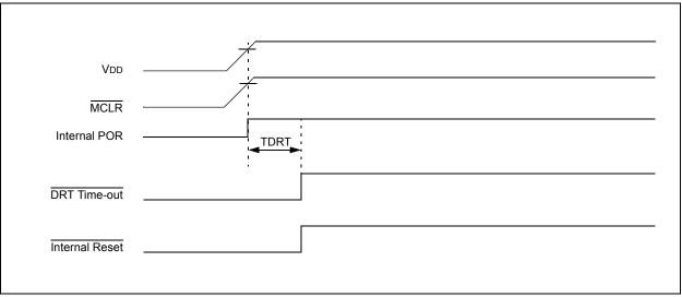
FIGURE 8-10: TIME-OUT SEQUENCE ON POWER-UP (MCLR TIED TO VDD): SLOW VDD RISE TIME
