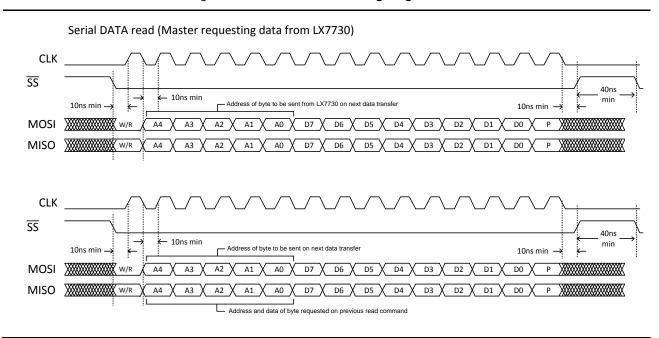
Figure 7 · Serial Data Read Timing Diagram
