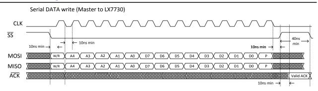
Figure 6 · Serial Data Write Timing Diagram
