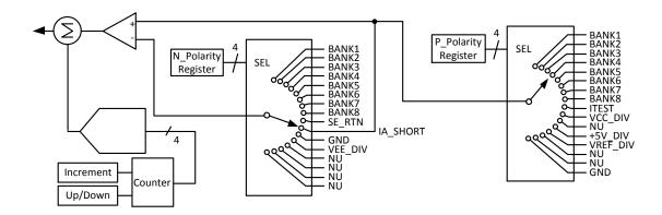
Figure 10 · IA Short IA Offset Adjust Test Configuration
