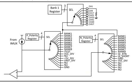
Figure 11 · Non-Inverting AMUX Continuity Check Test Configuration
