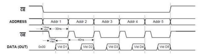
Figure 9 · Parallel Data Transfer Timing Diagram for Successive Data Transfers
