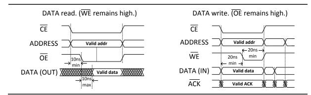
Figure 8 · Parallel Data Transfer Timing Diagram
