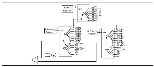
Figure 12 · Inverting AMUX Continuity Check Test Configuration
