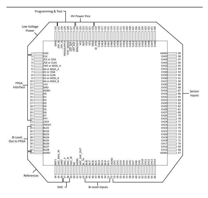
Figure 2 · Pinout
