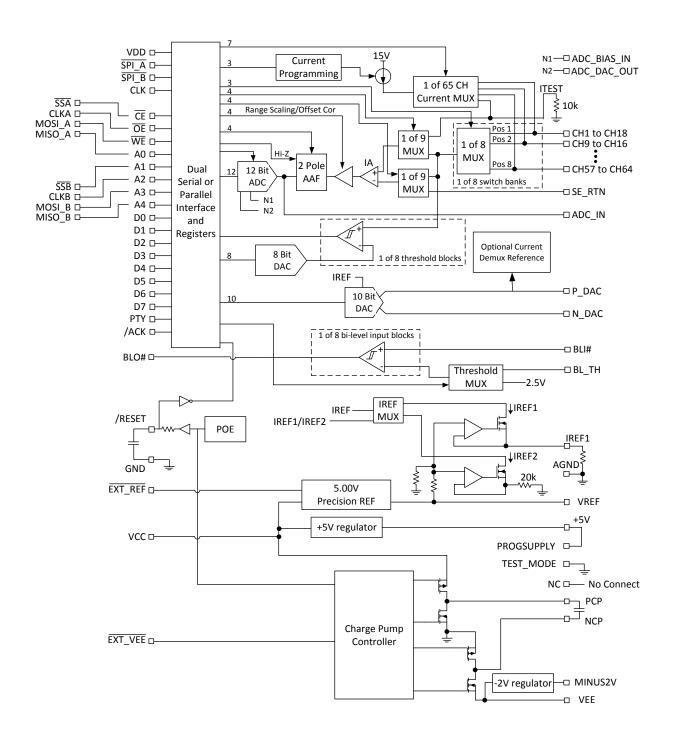
Figure 3 · LX7730 Top Level Block Diagram
