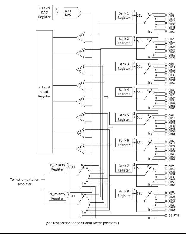
Figure 4 · LX7730 Sensor Multiplexer Expanded View Block Diagram
