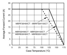
Figure 1. Forward Derating Curve Per Diode
