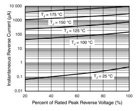
Figure 4. Typical Reverse Characteristics Per Diode
