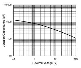
Figure 5. Typical Junction Capacitance Per Diode
