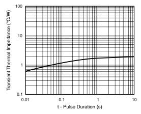
Figure 6. Typical Transient Thermal Impedance Per Diode
