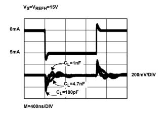
FIGURE 1. TRANSIENT LOAD REGULATION (SOURCING)
