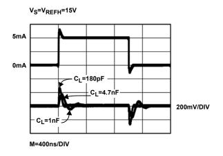
FIGURE 2. TRANSIENT LOAD REGULATION (SINKING)
