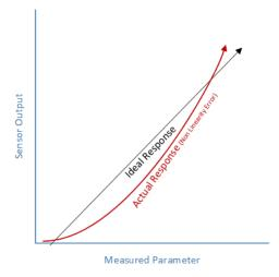
Sensors that are not linear over the measurement range require some curve-fitting to achieve accurate measurements over the measurement range. A common case requiring curve-fitting is thermocouples at extremely hot or cold temperatures. While nearly linear over a fairly wide range, they do deviate significantly at extreme temperatures.
