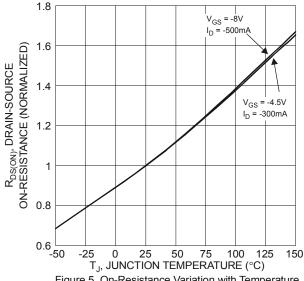
Figure 5 On-Resistance Variation with Temperature
