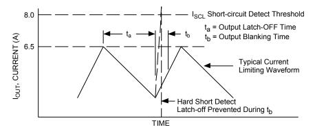
Figure 9. Active Current Limiting Detail
