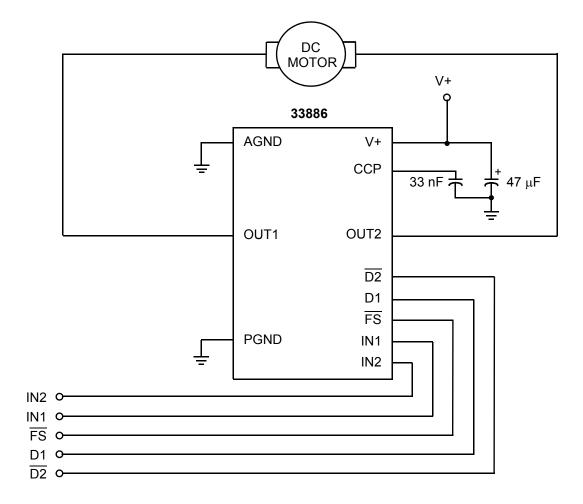
Figure 23. 33886 Typical Application Schematic
