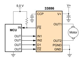
Figure 1. 33886 Simplified Application Diagram
