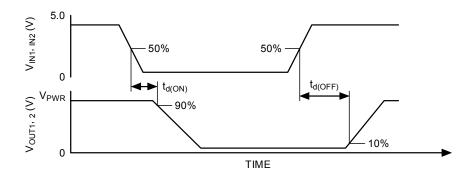
Figure 4. Output Delay Time
