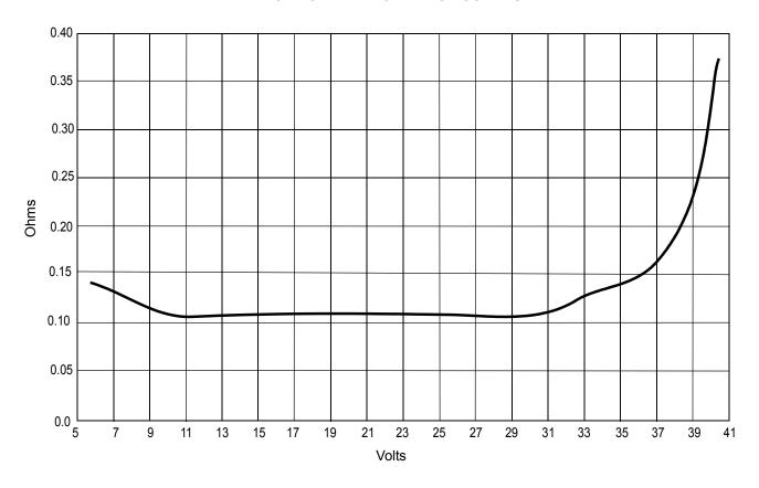
Figure 18. Typical High Side R<sub>DS(ON)</sub> Versus V+
