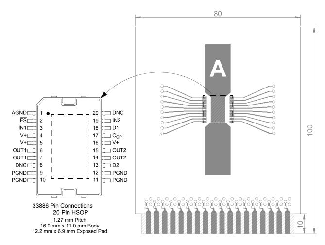
Figure 25. Thermal Test Board
