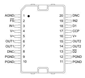
Figure 3. 33886 Pin Connections
