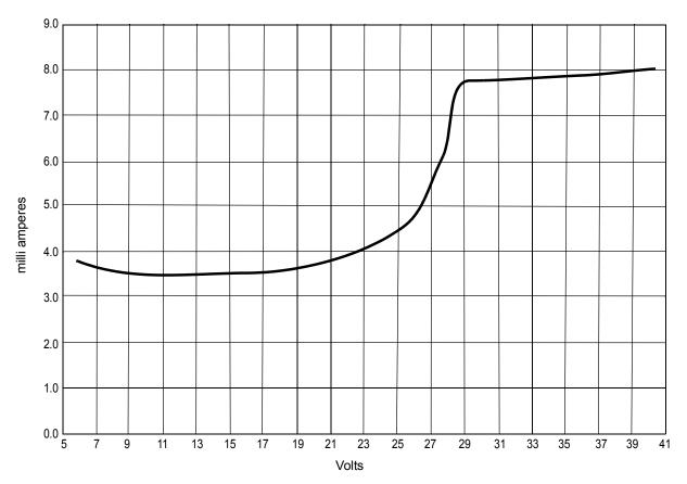
Figure 20. Typical Quiescent Supply Current Versus V+
