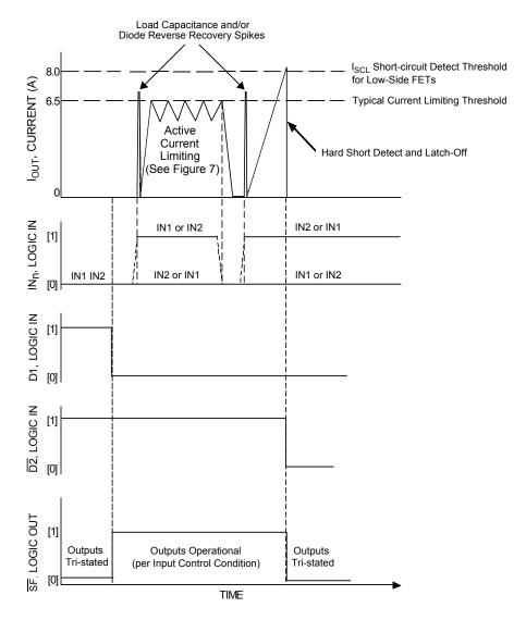
Figure 8. Active Current Limiting Versus Time
