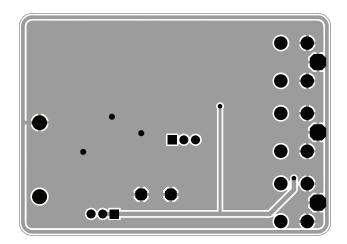
Figure 5: AAT3195 Evaluation Board Bottom Side Layout.
