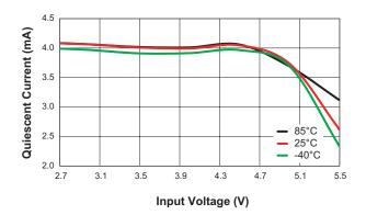
AAT3195-1 Current Matching vs. Temperature  $(V_{IN} = 3.6V)$
