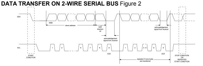
Figure 2 details how data transfer is accomplished on the 2-wire bus. Depending upon the state of the R/W bit, two types of data transfer are possible:
