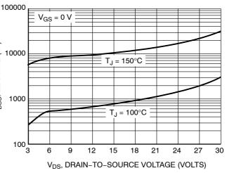
Figure 6. Drain-to-Source Leakage Current vs. Voltage
