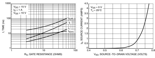
Figure 9. Resistive Switching Time Variation vs. Gate Resistance
