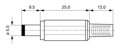
Cable diameter max. 4.0 mm
