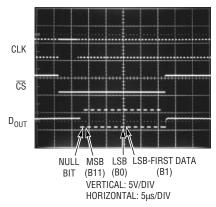
Figure 29. Scope Trace of the LTC1297 "Quick Look" Circuit Showing A/D Output 101010101010 (AAA<sub>HEX</sub>)
