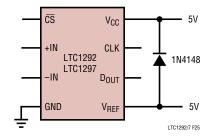
Figure 25. Separate V<sub>CC</sub> and V<sub>REF</sub> Supplies
