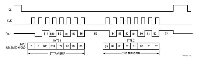
Figure 3. Data Exchange Between LTC1297 and MC68HC11
