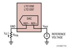
Figure 19. Parasitic Resistance in GND Pin
