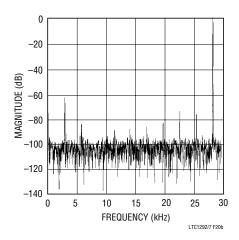
Figure 20b.  $f_{IN} = 28kHz$ ,  $f_{S} = 58.8kHz$ , SNR = 61.5dB
