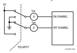
Load Circuit for  $t_{\mbox{\scriptsize dis}}$  and  $t_{\mbox{\scriptsize en}}$
