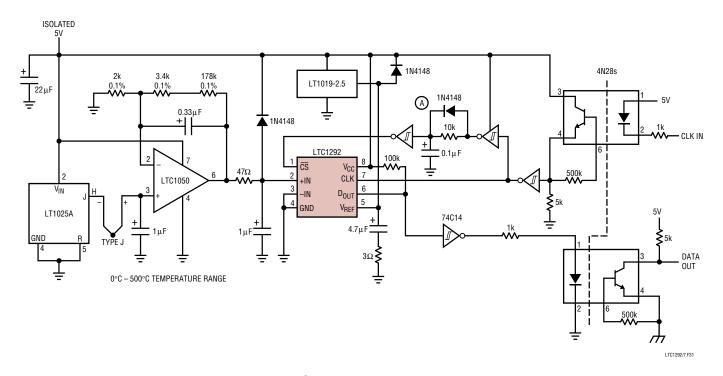
Figure 31. Opto-Isolated Temperature Monitor
