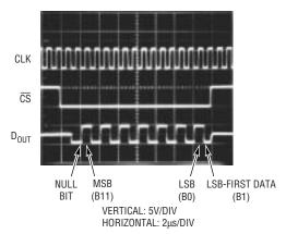
Figure 27. Scope Trace of the LTC1292 "Quick Look" Circuit Showing A/D Output 101010101010 (AAA<sub>HEX</sub>)
