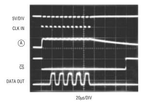
Figure 30. Opto-Isolated Temperature Monitor Digital Waveforms
