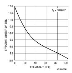
Figure 21. LTC1292 ENOB vs Input Frequency
