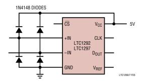
Figure 23. Overvoltage Protection with Clamp Diodes
