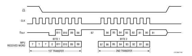
Figure 1. Data Exchange Between LTC1292 and MC68HC11
