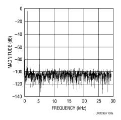
Figure 20a.  $f_{IN} = 1kHz$ ,  $f_{S} = 58.8kHz$ , SNR = 73.0dB
