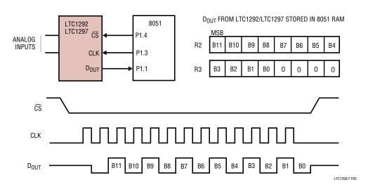
Figure 5. Hardware and Software Interface to Intel 8051 Processor
