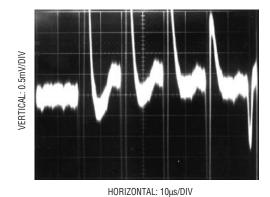
Figure 18. Poor Reference Settling Can Cause A/D Errors
