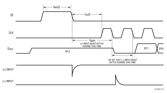
Figure 12. "+" and "-" Input Settling Windows for the LTC1297
