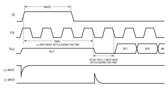
Figure 11b. Setup Time  $(t_{su}\overline{cs})$  Is Met for the LTC1292
