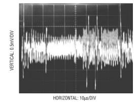
Figure 8. Poor V<sub>CC</sub> Bypassing. Noise and Ripple Can Cause A/D Errors
