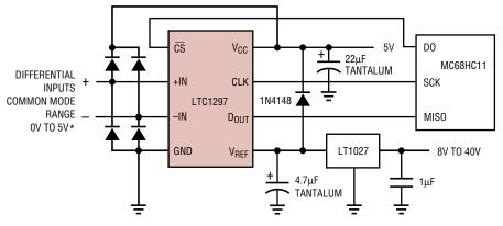
\*FOR OVERVOLTAGE PROTECTION LIMIT THE INPUT CURRENT TO 15mA PER PIN OR CLAMP THE INPUTS TO  $V_{CC}$  AND GND WITH 1N4148 DIODES. CONVERSION RESULTS ARE NOT VALID WHEN ANY INPUT IS OVERVOLTAGED ( $V_{IN}$  < GND OR  $V_{IN}$  >  $V_{CC}$ ). SEE SECTION ON OVERVOLTAGE PROTECTION IN THE APPLICATIONS INFORMATION.
