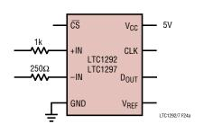
Figure 24a. Overvoltage Protection with Current Limiting Resistors
