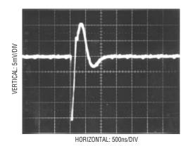
Figure 13. Adequate Settling of Op Amp Driving Analog Input
