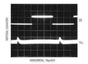
Figure 9. Good V<sub>CC</sub> Bypassing Keeps Noise and Ripple on V<sub>CC</sub> Below 1mV
