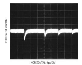
Figure 17. Adequate Reference Settling (LT1027)
