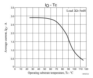
Overheating current control functions to prevent driver failure if a motor lock malfunction occurs.
