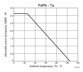
The package power dissipation, PdPK, refers to the internal average power dissipation, Pd, permissible if used without a heat sink
