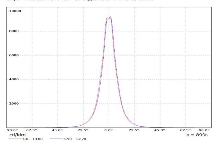
Luminaire: Ledil FCA12104\_IRIS\_(NVSW319AE) Lamps: 1 x Nichia\_NVSW319AE\_126.239Im@250mA\_P=0.729675W\_I=0.25A
