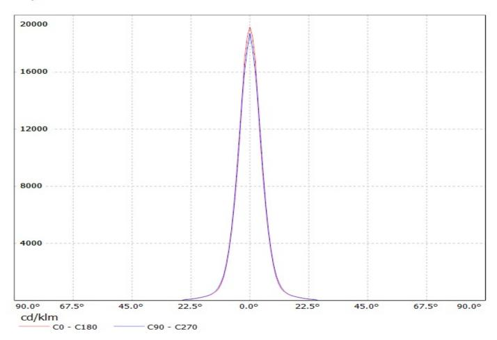
Luminaire: LEDil Oy FCA12104\_IRIS\_(XM-L2) Efficiency=86% Lamps: 1 x Cree XM-L2 (XMLBWT-0-7B4-T30-0L-0001) 91Im @ 250mA CCT=3200K P=0.7W I=250mA
