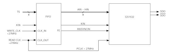
Figure 3-3: DVB-ASI FIFO Implementation using the GS1532
