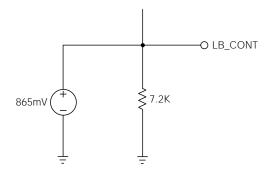
Figure 2-7: PLL Loop Bandwidth Control
