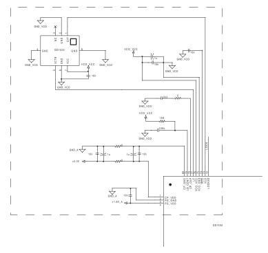
Figure 3-4: Typical Application Circuit using GO1525
