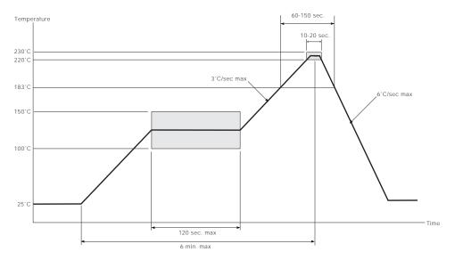
Figure 2-1: Standard Eutectic Solder Reflow Profile
