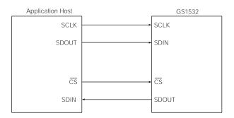
Figure 3-6: Gennum Serial Peripheral Interface (GSPI)
