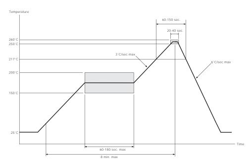
Figure 2-2: Maximum Pb-free Solder Reflow Profile (Preferred)
