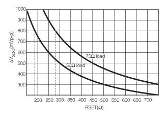
Figure 3-5: Serial Digital Output Swing
