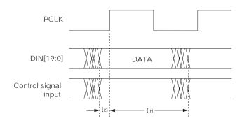
Figure 3-1: PCLK to Data Timing
