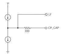
Figure 2-4: VCO Control Output & PLL Lock Time Capacitor
