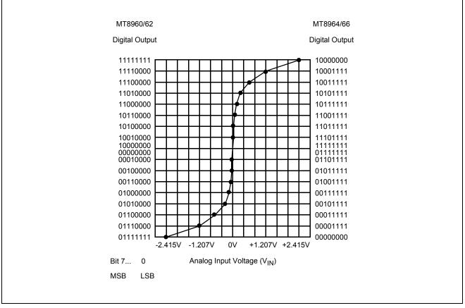
Figure 3 - µ-Law Encoder Transfer Characteristic
