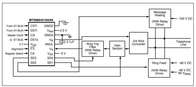
Figure 7 - Typical Use of the Special Drive Outputs
