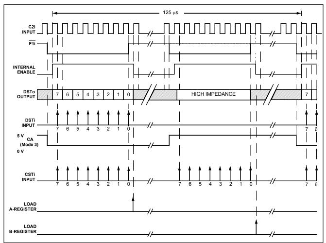
Figure 9a - Timing Diagram - 125  $\mu$ s Frame Period
