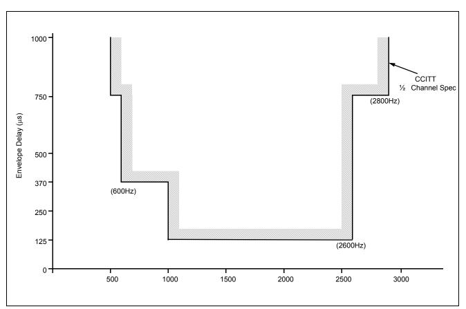
Figure 14 - Envelope Delay Variation Frequency
