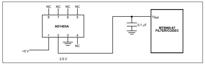
Figure 5 - Typical Voltage Reference Circuit
