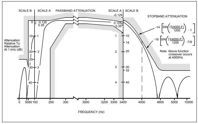
Figure 10 - Attenuation vs Frequency for Transmit (A/D) Filter
