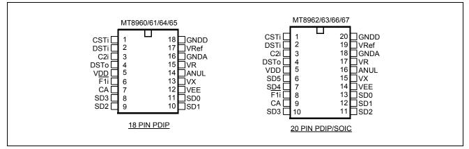
Figure 2 - Pin Connections
