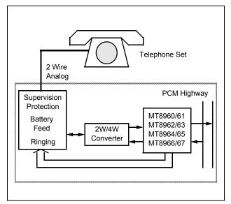
Figure 6 - Typical Line Termination
