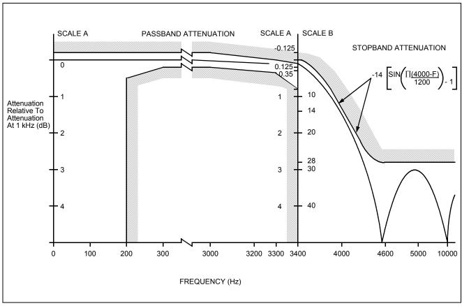
Figure 11 - Attenuation vs Frequency for Receive (D/A) Filter
