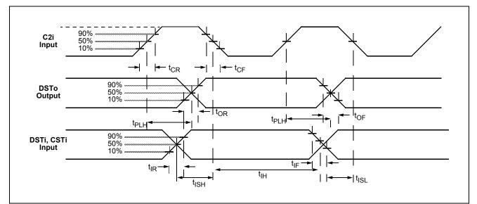
Figure 9c - Timing Diagram - Input/Output
