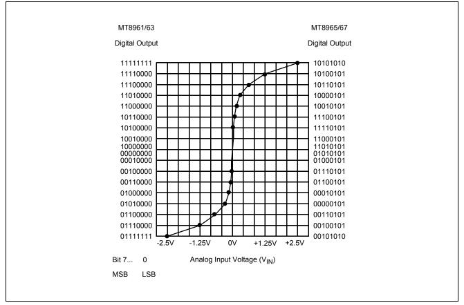
Figure 4 - A-Law Encoder Transfer Characteristic
