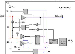
Figure 13 Circuit connected to VINS pin
