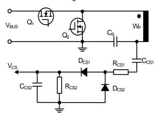
Figure 10 Current sense circuit
