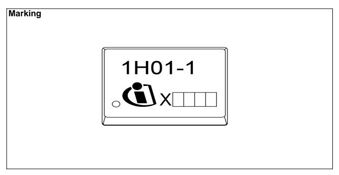
Figure 16 Marking for ICE1HS01G-1
