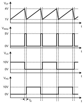
Figure 4 Oscillator waveforms
