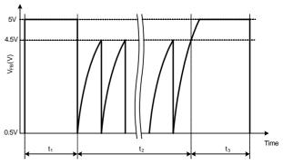
Figure 12 FB voltage waveform during over load protection
