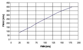
Figure 7 Fmax versus Fmin during normal operation
