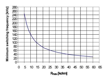
Figure 5 FMIN versus R<sub>FMIN</sub>
