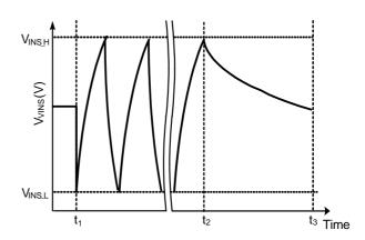
Figure 14 VINS voltage waveform during blanking time after OLP and before IC restarts
