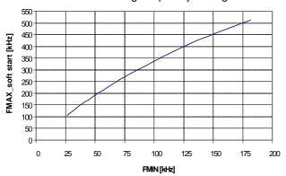
Figure 8 Fmax\_ss versus Fmin during soft start
