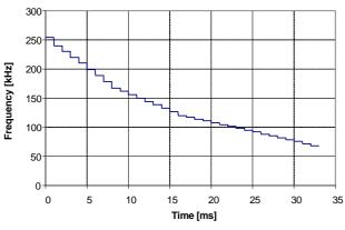
Figure 9 Switching frequency during softstart when R<sub>FMIN</sub>=22kohm
