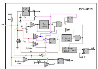
Figure 11 Circuit connected to FB pin
