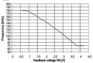
Figure 6 Switching frequency versus V<sub>FB</sub>
