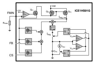
Figure 3 Simplified oscillator circuit
