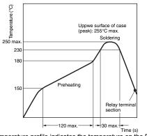
(The temperature profile indicates the temperature on the PCB.)
