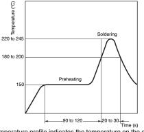
(The temperature profile indicates the temperature on the circuit board.)
