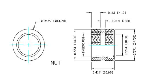
M12 FEMALE - CABLE MOUNT - SOLDER CUP - 5 POS.
