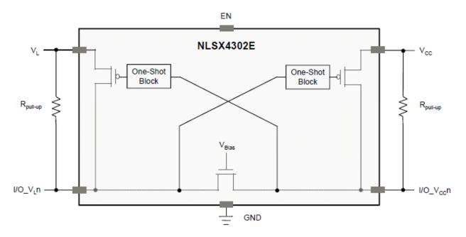
Figure 1. Block Diagram (1 I/O Line)
