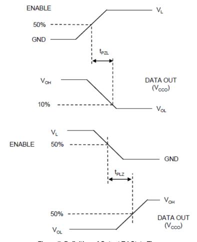
Figure 7. Definition of Output Tri-State Times
