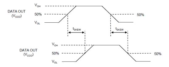
Figure 6. Definition of Output Skew
