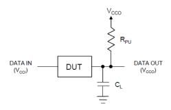
Figure 3. AC Test Circuit
