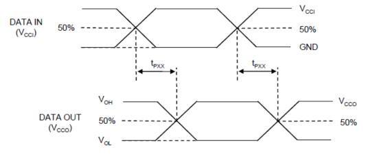
Figure 4. Propagation Delays and Tri-State Measurements
