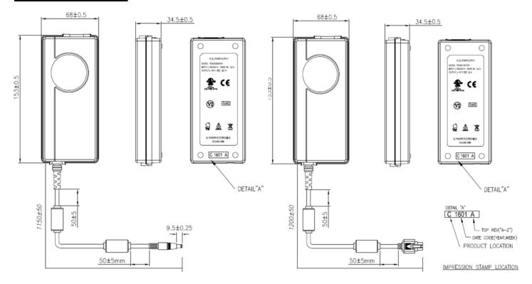
15V through 24V Models: 2.5 x 5.5 x 9.5mm Barrel Connector, center positive. 12V Models: Output Connector: 6 pin Molex 39-01-2060 or equiv. Pins 1, 4 = (+), pins 3, 6 = (-), pins 2, 5 = NC
