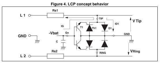
*Figure 4* shows the classical protection circuit using the LCP crowbar concept. This topology has been developed to protect the new high voltage SLICs. It allows to program the negative firing threshold while the positive clamping value is fixed at GND.
