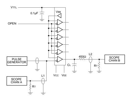
Figure 2. AC Test Circuit for 15pF Loading
