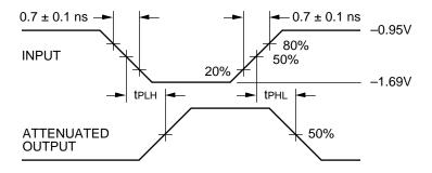
Figure 1. Propagation Delay
