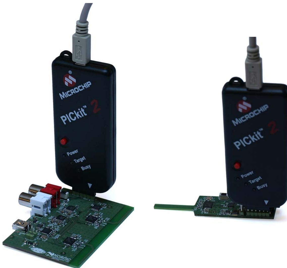
Figure 3. Receiver board and microphone setup with PICkit2™
