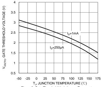
Figure 8. Gate Threshold Variation vs. Temperature
