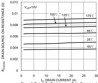
$\rm I_D,\,DRAIN\,CURRENT$  (A) Figure 5. Typical On–Resistance vs. Drain Current and Temperature
