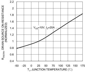
Figure 6. On-Resistance Variation with Temperature
