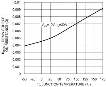
Figure 7. On-Resistance Variation with Temperature
