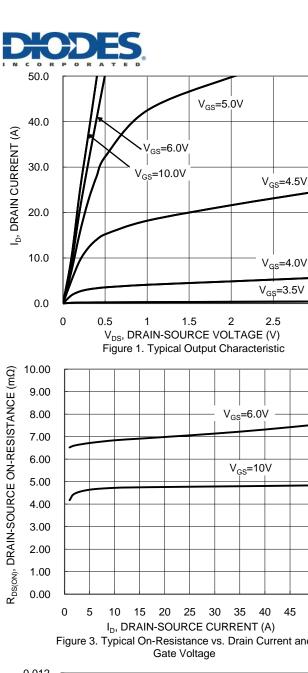
Figure 3. Typical On-Resistance vs. Drain Current and
