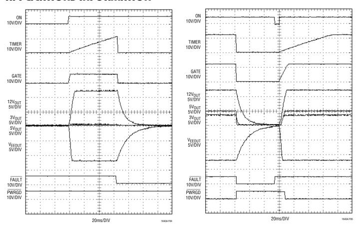
Figure 4. Power-Up into a Short on 3.3V Output
