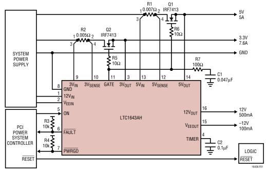
Figure 1. Typical PCI Application
