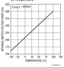
V<sub>EE</sub> Internal Switch Voltage Drop vs Temperature
