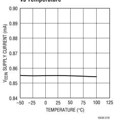
5V<sub>IN</sub> Supply Current vs Temperature
