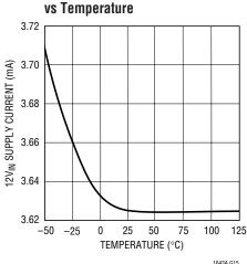
V<sub>EEIN</sub> Supply Current vs Temperature
