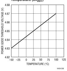
Power Good Threshold Voltage vs Temperature (3V<sub>OUT</sub>)
