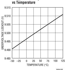
5V<sub>IN</sub> Undervoltage Lockout vs Temperature
