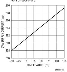
3V<sub>IN</sub> Supply Current vs Temperature
