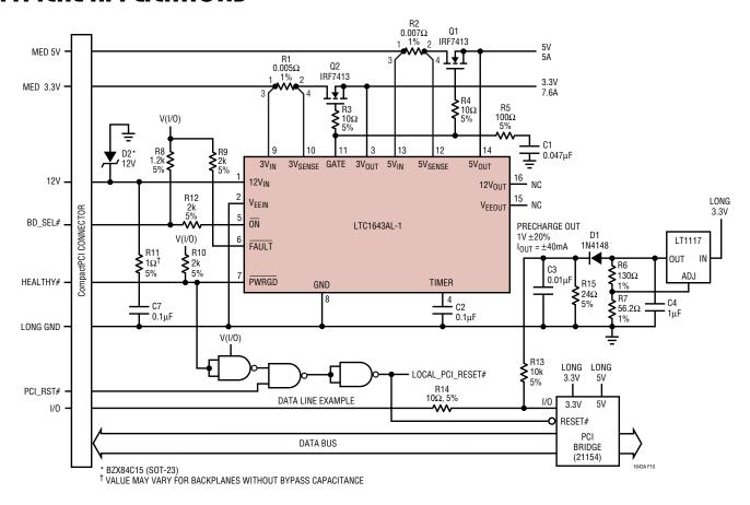
Figure 10. CompactPCI Application without  $\pm 12V$  Outputs
