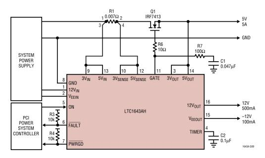
Figure 9. System Without 3.3V Supply
