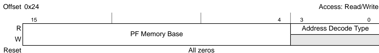
Figure 17-79. PCI Express Prefetchable Memory Base Register
